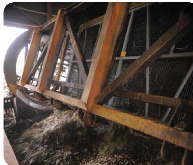
Cane tipper, emptying transported cane into the milling process at Farleigh Mill, Mackay.
